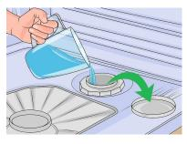
If a new machine, check for water and fill reservoir if empty.
