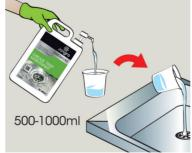
Pour 500 -1000ml into the drain or sink flowing to the trap.
